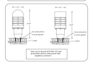
A decorative garden light with a fully shielded lamp providing symmetrical light distribution with no glare and meeting Dark Sky criteria. Designed to house different options of energy saving compact fluorescent, metal halide and high pressure sodium lamps Developed to compliment the Texas garden light, Texas bollard and Texas pillar light. For use in various applications including entrances, gardens and pathways.
