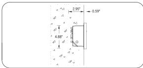
A range of rectangular and square wall recessed luminaires, with an indirect optical system, offering high vandal resistance. Suitable for indoor or outdoor applications. The recessed LED eliminates all discomfort glare as light is directed to the ground providing illumination where it is needed and
